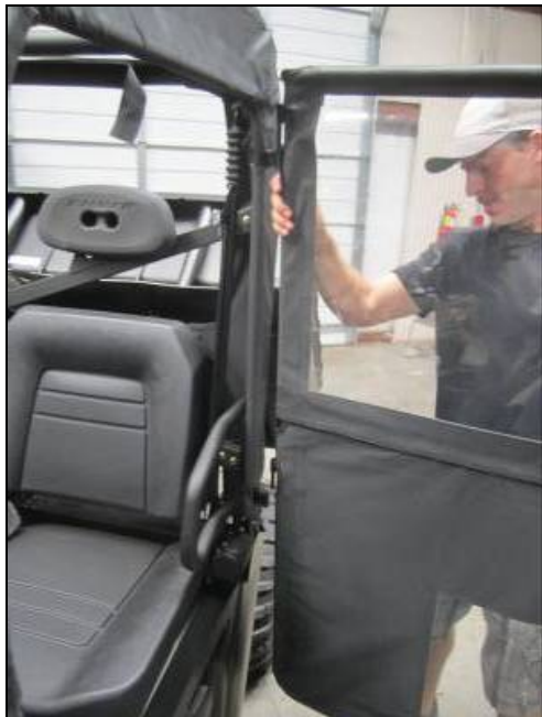
14. Mount the doors by guiding the pins in the back of the door frame onto the hinge barrels along the Rear Hangar Bar.
